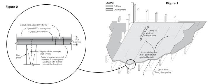
Figures 1 & 2 – Typical Subfloor/Underlayment Detail (Not to Scale)
