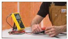
1 Before the heating cable is removed from the spool, conduct the first set of required tests and record values in the heating cable tests log (page 39). If a break or damage is detected during the tests, return the heating cable to the original place of purchase.
