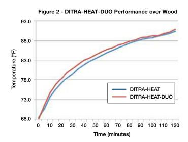
DITRA-HEAT-E-HK heating cables were spaced at three studs in all of the above tests.
