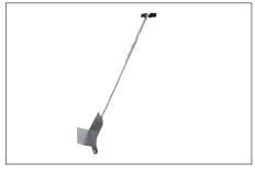
When using the DITRA-ROLLER, place a weight (e.g., bags of mortar/grout or box of tile) not to exceed 75 lbs on the DITRA-ROLLER shelf. Slowly move the roller from one end of the matting to the other, slightly overlapping successive passes
