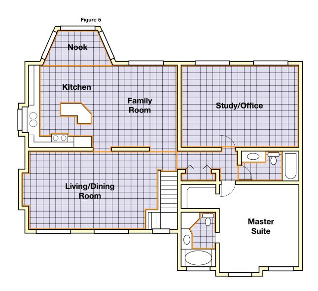
Schluter-Systems understands that the tile setter must take into account the needs of his or her client in determining the placement of movement joints in a tile installation. For example, a client may not wish to interrupt a continuous tile field that spans multiple rooms. However, as indicated by the orange lines above, there are ways to meet industry guidelines that will serve to provide the client with a durable installation that remains aesthetically pleasing.
